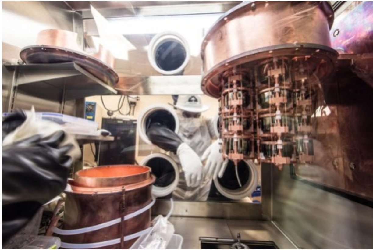
Loading of ^{enr}\text{Ge} in Cryostat 1
