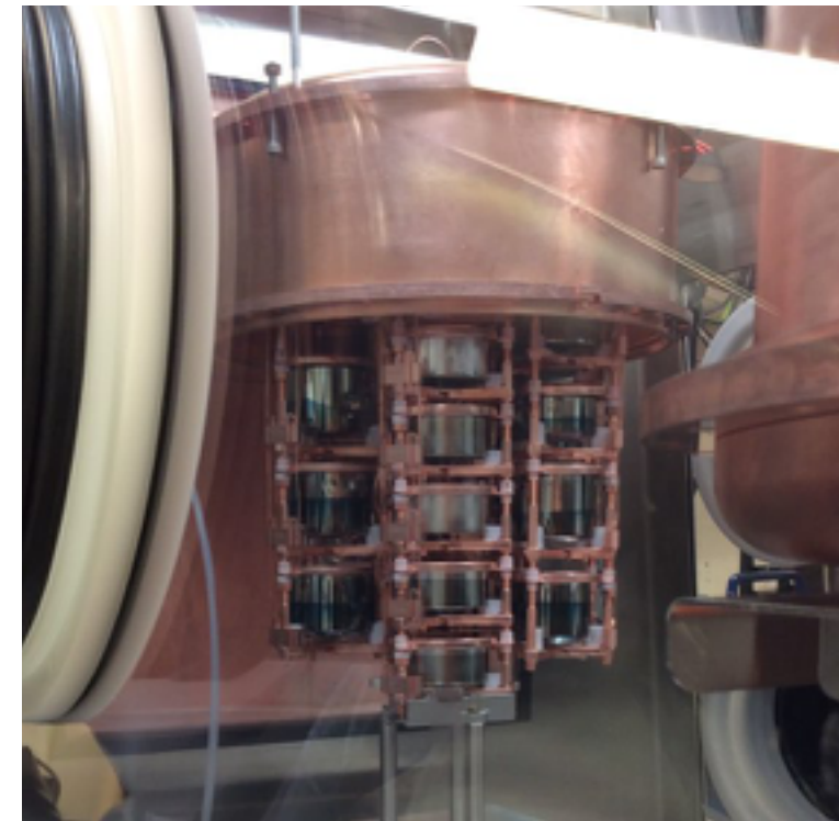
Loading of ^{enr}\text{Ge} in Cryostat 2
