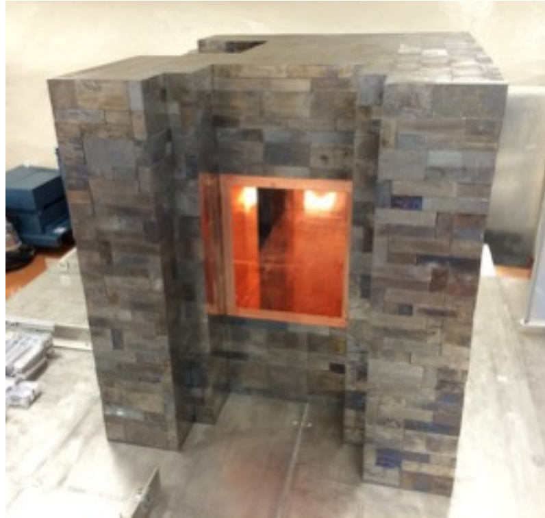
Pb and outer Cu shield
